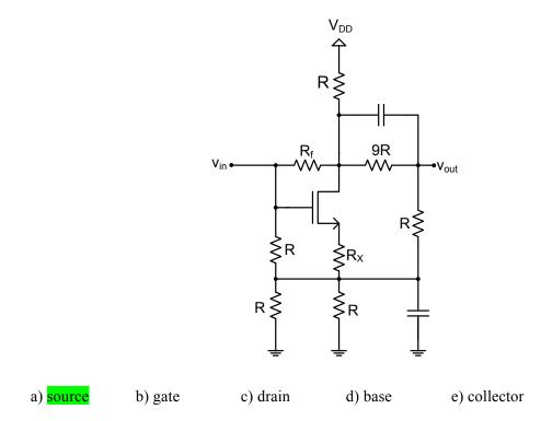
8. Find the voltage gain (in absolute value) of the amplifier in the previous problem,  $v_{out}/v_{in}$ , if  $g_m = 1 \text{ mA/V}$  for the MOSFET,  $R = 11 \text{ k}\Omega$  and  $R_X = 100 \Omega$ . Assume that all capacitors are very large with negligible impedance at signal frequencies. Also assume that  $R_f$  is a *very* large resistor.
