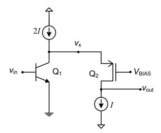
18. Find the output resistance of the amplifier (in  $M\Omega$ ).
