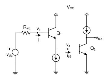
11. Find the gain of the CE stage,  $v_{out} / v_x$ .
