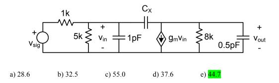
6. In the circuit of the previous problem, and after using Miller's theorem, the total capacitance on the input side of the circuit was found to be 120 pF. Find the value of the capacitor  $C_X$  (in pF). Assume  $g_m = 4 \text{ mA/V}$ .
