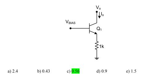
10. Find the output resistance (in M $\Omega$ ) of the current source in the previous problem. For the BJT,  $\beta = 100$ , and the Early voltage is 50 V. V<sub>BIAS</sub> is a pure DC source.
